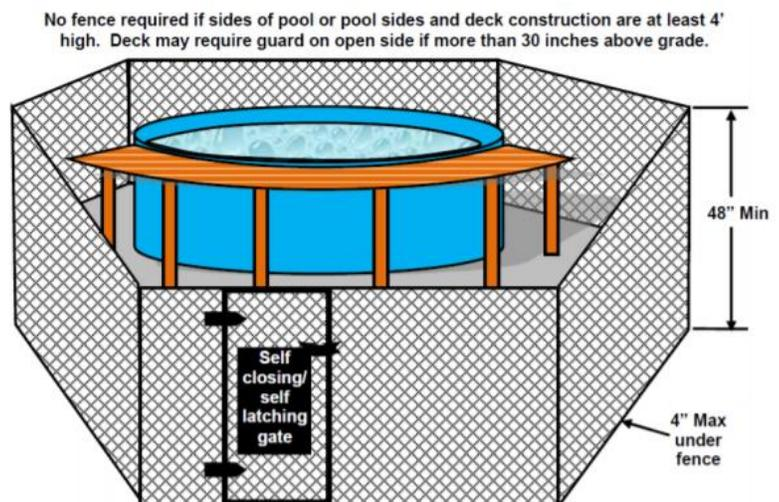
**305.2.2 Openings.** Openings in the barrier shall not allow passage of a 4-inch-diameter sphere.
